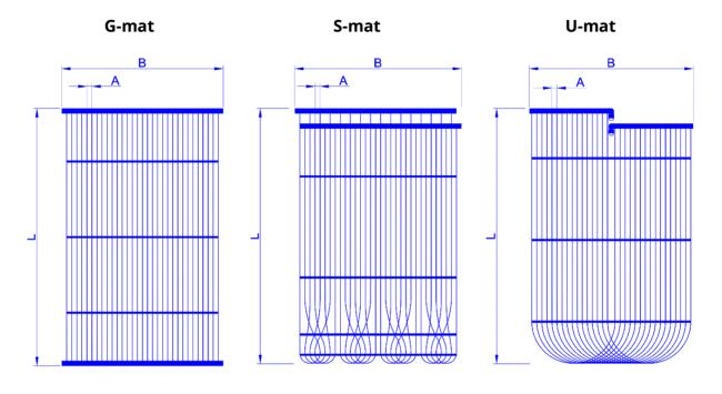
capillary tube 3,4 x 0,55 mm, round mat distributor pipe 20 x 2,0 mm
